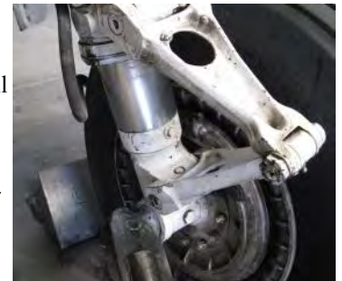
The main landing gear struts will be disassembled and the shiny surfaces polished for smoother taxi operation
