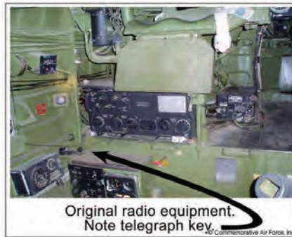
Radio Operator's position, below the turret gunner seat. Above the telegraph key is the large Collins ART-13 "Auto-tune" transmitter.
