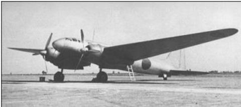
Ki-77, was a Japanese long-distance record aircraft with a remarkably slim fuselage and finely tapered wide-span monoplane wings. Two were built to set long distance records. The first was lost on an attempt from Japan to Europe in 1943. The second set a closed course long distance record of 16,435 Kilometers on July 2, 1944.
